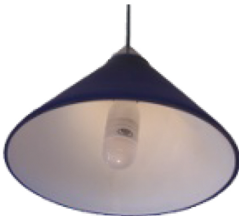
Competitor's LED bi-pin is ineffective in reflector as optical centre is significantly displaced from optimal position
